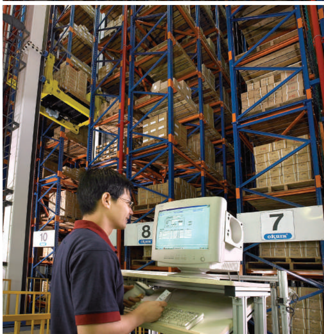
30 meter height, ASRS (Automated Storage & Retrieval System)
