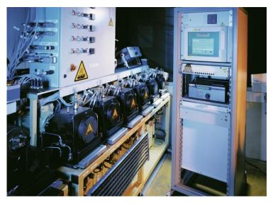
Endurance testing of radial bearings: A rating life test stand at Schaeffler's research and development center in Herzogenaurach. The testing method has earned the company Germanischer Lloyd's prestigious seal of approval.
